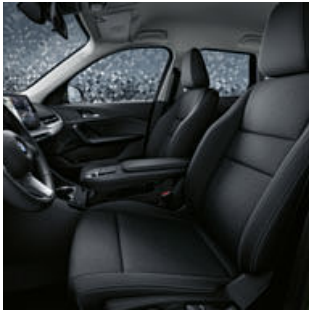
The standard seats for driver and front passenger offer a great deal of comfort. The seat height, fore/aft position, backrest angle and head restraint height can be adjusted manually. A map pocket is located on the rear panel. The seat belt buckle tensioner and belt force limiter also increase safety.
