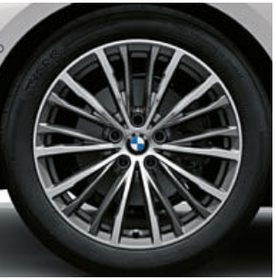
18" light alloy wheels Multi-spoke style 781 Bicolour Ferric Grey with mixed tyres, gloss-lathed, front 7.5J x 18 with 225/45 R18 tyres, rear 8.5J x 18 with 255/40 R18 tyres.
