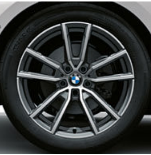
18" light alloy wheels V-spoke style 780 Bicolour Orbit Grey with mixed tyres, gloss-lathed, wheel size front 7.5J x 18 with 225/45 R18 tyres, wheel size rear 8.5J x 18 with 255/40 R18 tyres.
