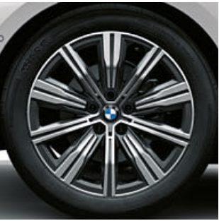
18" light alloy wheels Double-spoke style 782 Bicolour Jet Black, gloss-lathed, wheel size 7.5J x 18 with 225/45 R18 tyres.
