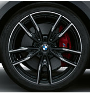
19" M light alloy wheels Double-spoke style 792 M Bicolour Jet Black with mixed tyres and runflat tyres, gloss-lathed, front 8J x 19 with 225/40 R19 tyres, rear 8.5J x 19 with 255/35 R19 tyres. 4
